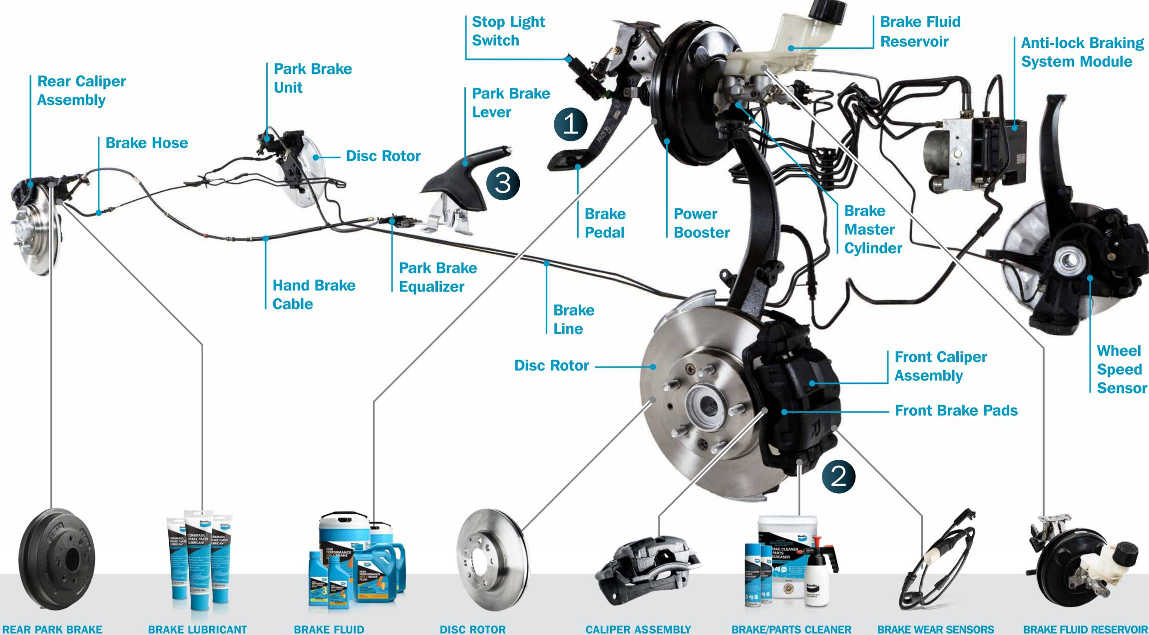
The park brake system can operate through the rear disc pads or a shoe and drum brake system. The park brake should be regularly checked and/or adjusted to ensure correct operation and the brake linings should not be allowed to wear past the manufacturer's recommendations.
